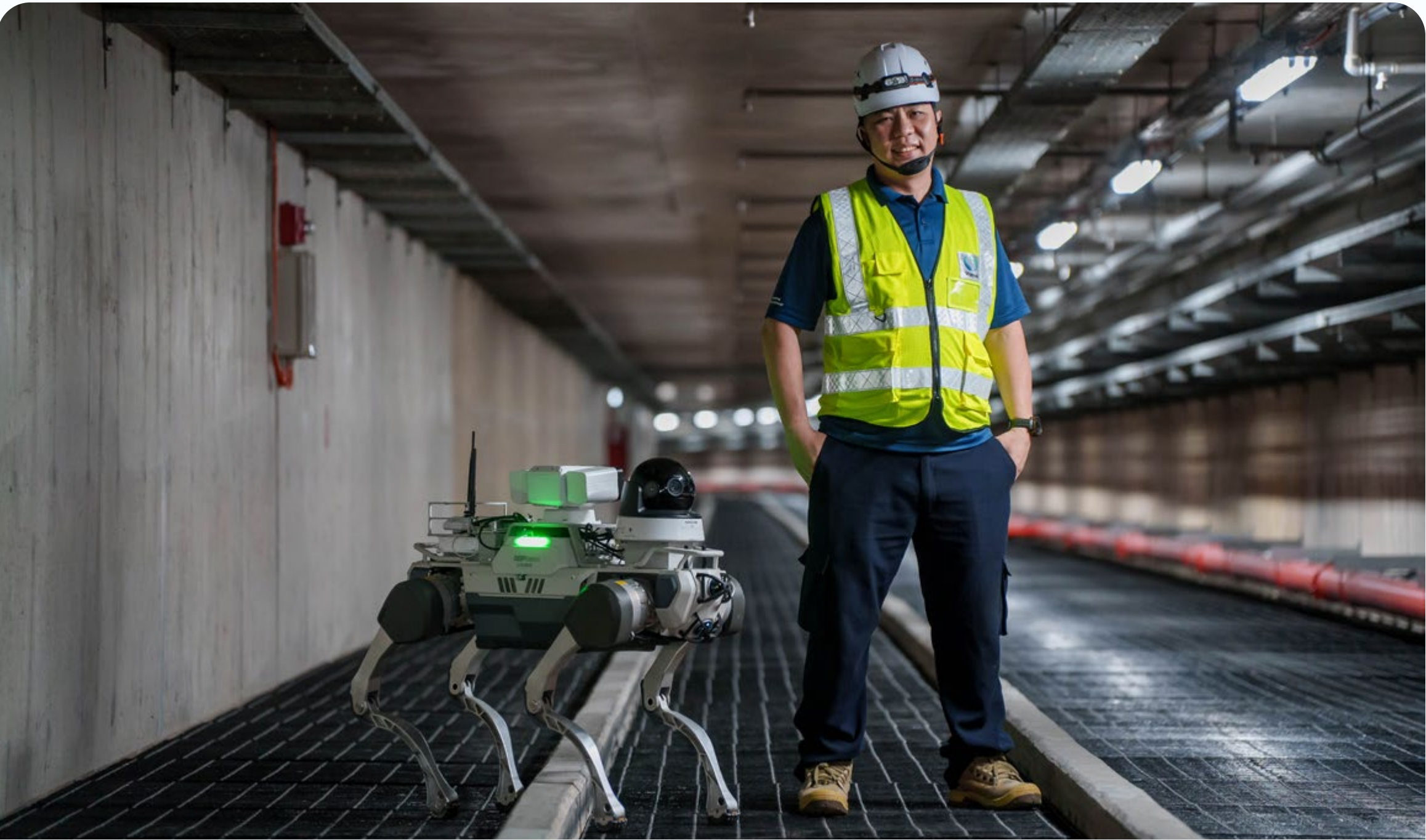
Spock, a robotic dog, assists our facility management team in preventative potential hazard identification and inspection
