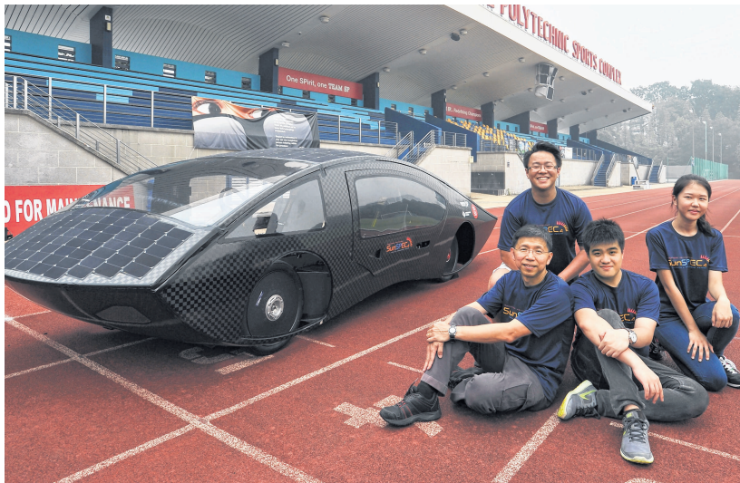
(Clockwise from bottom left) Team manager and senior lecturer Steven Chew with students Daniel Quick, 20; Lee Sunho, 21; and Cheong Yong Quan, 21, who are driving the Singapore Polytechnic team's black SunSPEC4, a 220kg carbon-fibre car lined with solar cells. The polytechnic is taking part in the World Solar Challenge, a 3,000km endurance race from Darwin to Adelaide, from Oct 18 to 25. PHOTO: LIM YAOHUI FOR THE STRAITS TIMES
