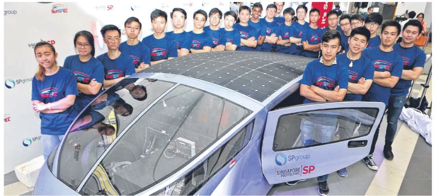
Singapore Polytechnic is entering the World Solar Challenge for the third time. Its SunSPEC5 solar-powered car was 20 months in the making and has a top speed of 100kmh. Hopes are high that this year's race in the advanced Cruiser Class category will go smoothly. PHOTO: SP GROUP
