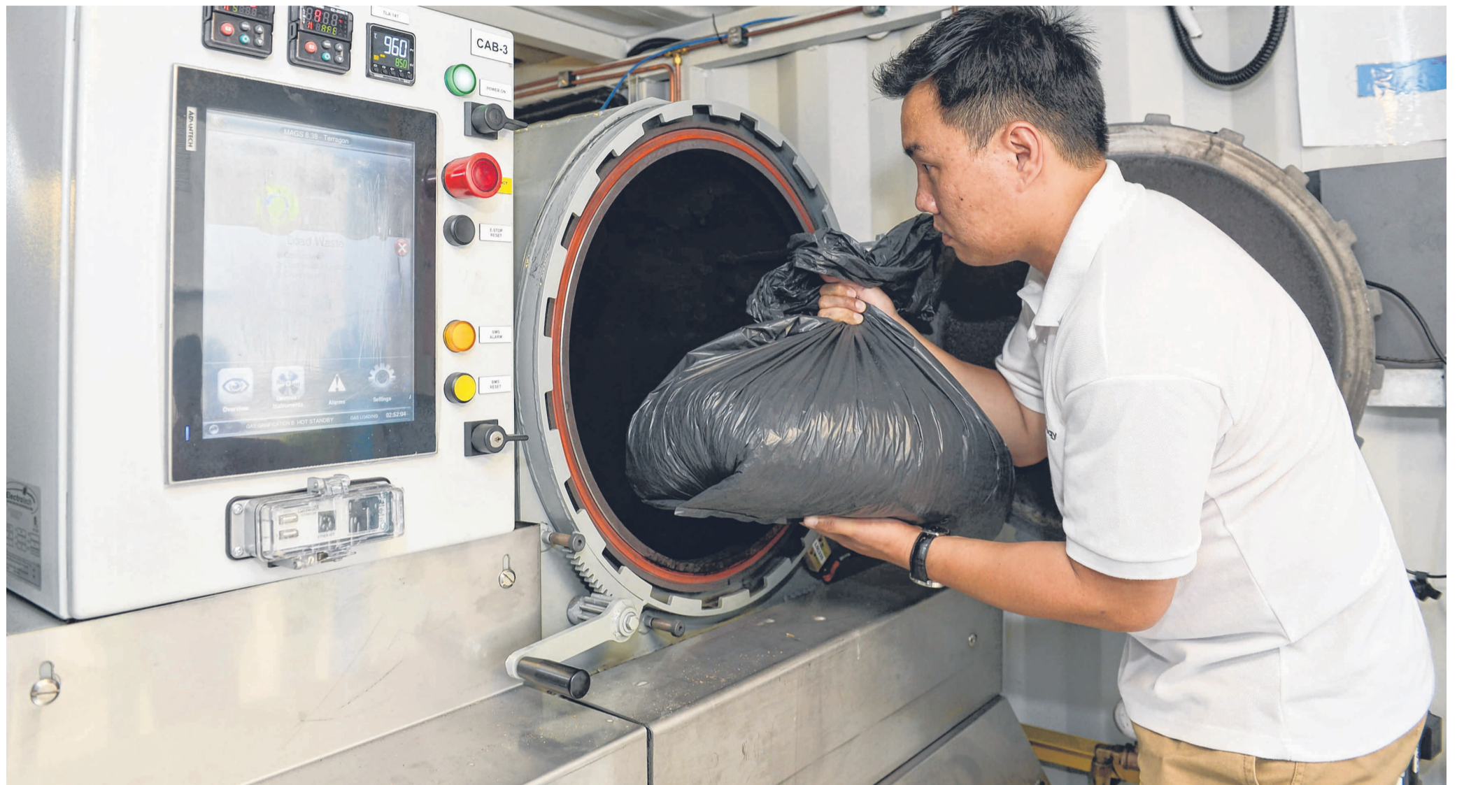
Mr Dex Ng, assistant director for conservation and environmental sustainability at Gardens by the Bay, demonstrating the disposal of trash into the gasification system. The system, created by SP Group, began operating last month and will run as a pilot project till May 2021. It will help to reduce Singapore's reliance on the Pulau Semakau landfill, which is expected to be filled by 2035. ST PHOTO: SHINTARO TAY
